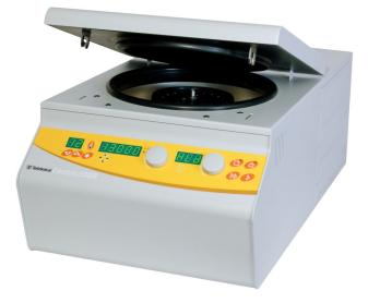
**Centrifuge CENTRIC 200R** (mark R means with refrigerating system) is universal laboratory centrifuge, designed for use in medical, industrial and scientific laboratories for separating substances with different relative densities by centrifugal force. The maximum rotational speed of **16.200 RPM** gives the centrifugal force of **25.000** x g.
